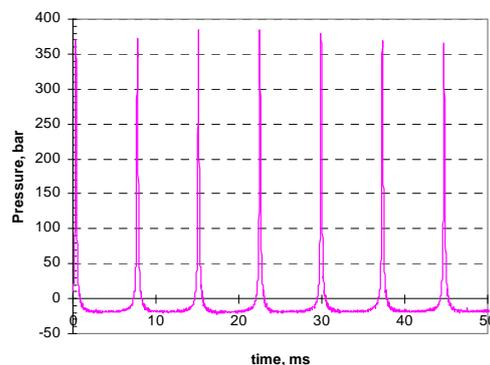
Figure 3. Pressure change in the single-chamber reactor during continuous syngas production:  $\phi = 3.6$ .
