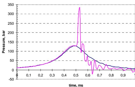
Figure 2. Influence of propane on the pressure change in the single-chamber reactor; dark blue line – without propane, purple line – with propane ( $\phi = 0.63$ ).
