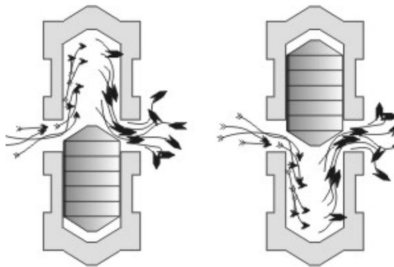
Figure 1. Operating principle of the pulsed compression reactor.
