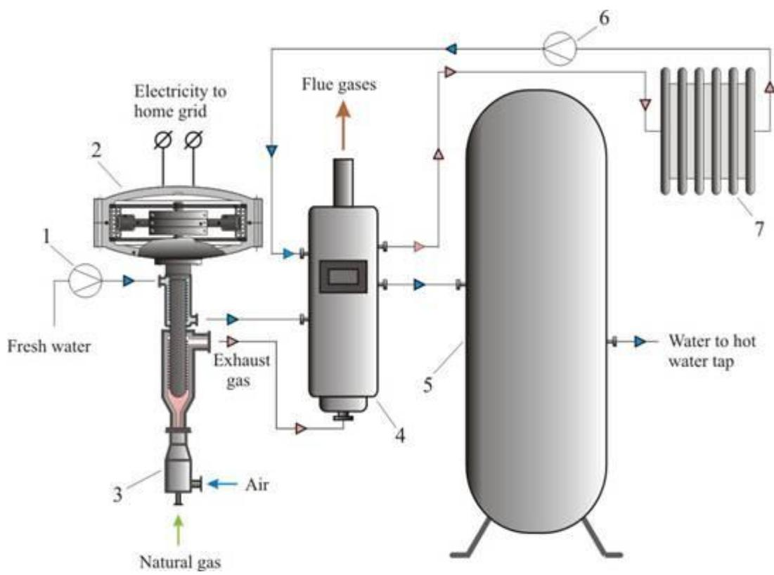
**Figure 2. Possible domestic micro-CHP installations**
