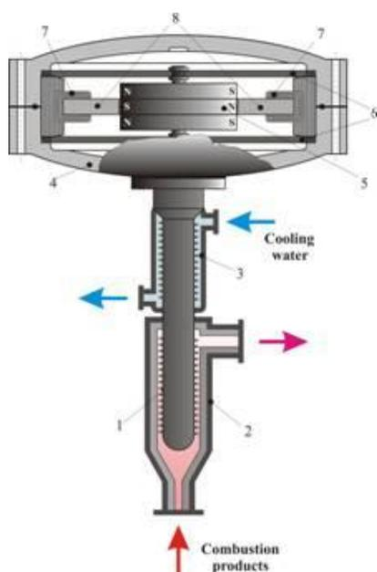
**Figure 1. Novel heat-to-electricity converter**
