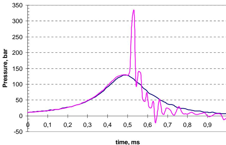
Figure 3. Influence of propane on the pressure change in the reactor; dark blue line – without propane, purple line – with propane ( $\phi = 0.63$ ).
