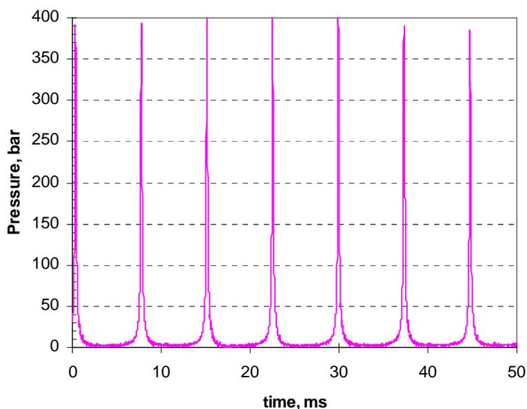
Figure 4. Pressure change in the reactor during continuous production of syngas ( $\phi = 3.6$ ).
