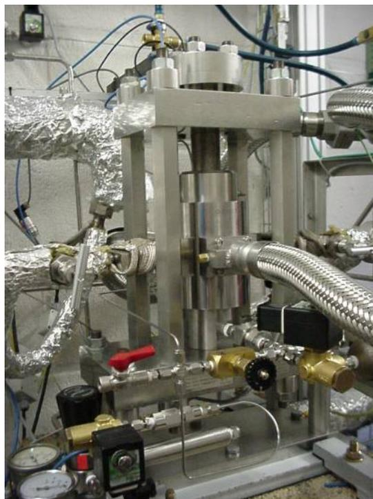
Figure 2. Double-chamber reactor placed inside massive frame.
