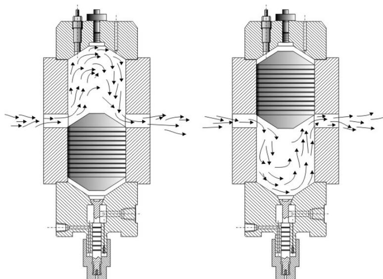
Figure. 1. Pulsed compression reactor. Two limiting positions of the reciprocating piston are shown.
