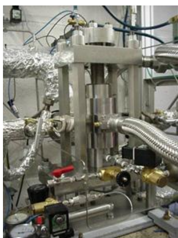
Figure 2. Double-chamber reactor placed inside massive frame
